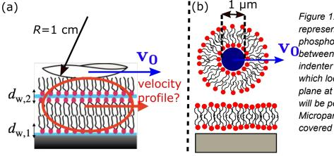
Figure 1: (a)Schematic representation of a phospholipid trilayer sheared between a rigid spherical indenter (diameter~5 cm) for which localization of the sliding plane at low and high velocities will be performed. (b) Microparticles (1 µm size) covered with a lipid bilayer.
