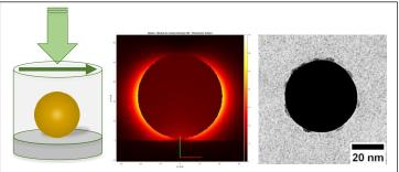
**Figure**: (Left) Schematic view of a metal nanoparticle in the photopolymerization under irradiation. (Center) Simulated electro-magnetic field around the nanoparticle showing the exaltation and confinement of the field near the nanoparticle surface. (Right) TEM image after polymerization showing single macromolecules grafted at the surface of the metal nanoparticle.
