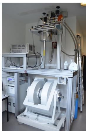
Figure: (Left) Optical microscope picture of a typical propagating spin-wave spectroscopy device, where a pair nano-antennae (in white) allows one to excite and detect spin-waves with a wavelength of about 1 μm. (Right) Photograph of the experimental set-up essentially composed of an electromagnet (bottom), a cryostat (top) and a microwave network analyzer (top left).
