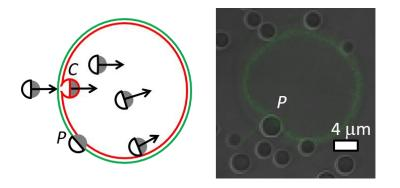
Figure 1 : (left) Sketch of Active Janus colloids completely C or partially P engulfed by a lipid membrane. (right) Microscopy image of colloids interacting with a lipid vesicle.
