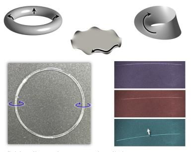
In our lab, the ICS, we have recently invented and created the first prototypes of novel, ultra-light, miniature motors consisting of only a single polymer fiber. The idea behind our invention is to prestrain a fiber, generate an embedded zero energy mode within the material and drive it as an internal wheel and active motor. Based on this "wheel within" principle we can now transform virtually any polymer fiber (from
