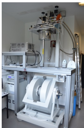
Figure: (Left) Optical microscope picture of a typical propagating spin-wave propagation device. The pair of spin-wave nano-antennae (in white) allows one to excite and detect spin-waves with a wavelength of about 1\mu\text{m} . (Right) Photograph of the experimental set-up showing the electromagnet (bottom), the cryostat (top) and the microwave network analyzer (top left).
