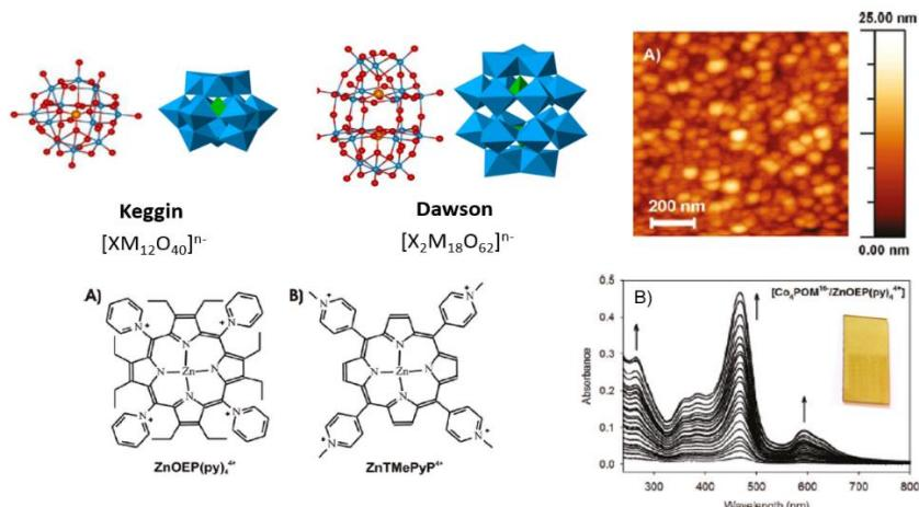
Right: structures of POMs and of tetracationic porphyrins. Left: tapping mode AFM topography and UV-visible absorption spectra of [POM/ZnOEP(py)<sub>4</sub><sup>4+</sup>]<sub>n</sub> films (onto quartz) with different numbers of deposition cycles (n).
