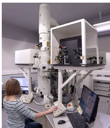
Figure 1 : New ultrafast transmission electron microscope at the IPCMS. It combines the vertical column of the electron optics with an extended periphery for the laser optics.
