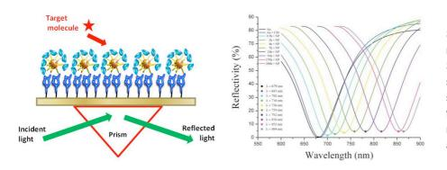
Schematic representation of an SPR biosensor and shift of the SPR signal as function of the structure of nanoparticle assembly
